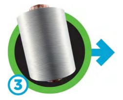
polyester chips are extruded into recycled polyester yarn or monofilament
